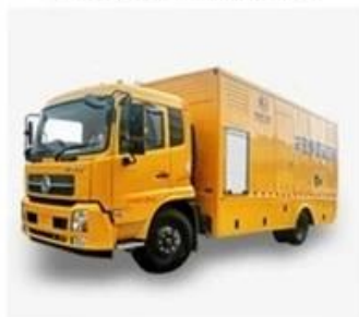
EMERGENCY POWER SUPPLY VEHICLES
