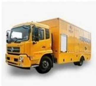
EMERGENCY POWER SUPPLY VEHICLES
