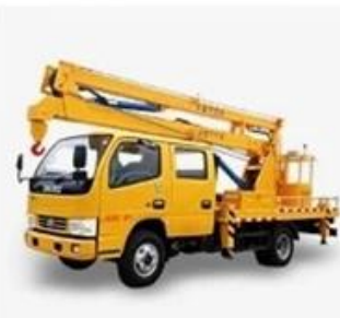
AERIAL WORK TRUCKS
